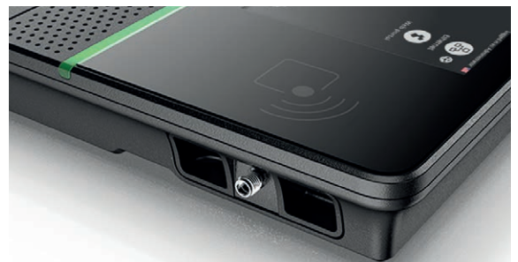
Antenna connector (SMA female). Maximun antenna gain: +8dBi
