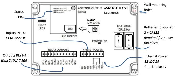
Step 2: Power, batteries and connecting to your devices
