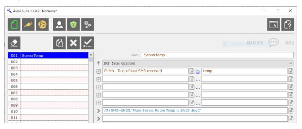
Avior is waiting for someone to send the SMS with the word "temp" and on receipt it will send a SMS back to the last number (\$N23) and send the message with the analogue value \$A12 embedded within.
